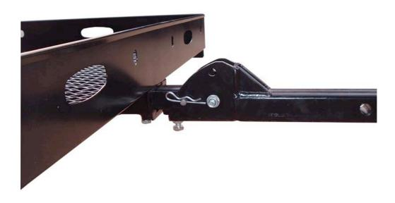
Step.2 Insert four 3/8"x7/8" bolts on the bottom of your carrier tube. Tighten bolts firm with a wrench. See the figure.
