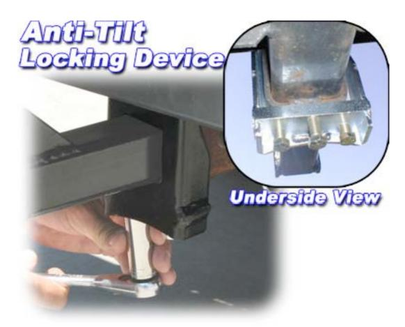
Next loosen the bolts on the anti-tilt lock bracket. (There should be grooves where the bolts were tightened against the hitch receiver)
