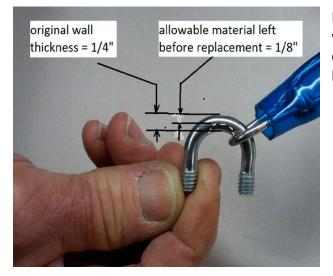
Note: For clarity, the seat u-bolt is shown without the seat. Also, although just one end of the chain is shown above, both ends would have to be inspected.
