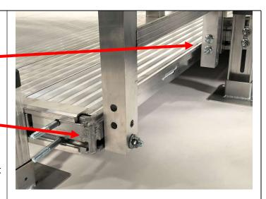
3e. The picture to the right shows the universal bracket assembly used for the vertical picket handrail square post coming onto the platform – it is assembled using a 2.5" universal bracket and two 3/8"-16 x 5" bolts.
