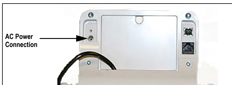
Figure 2-6. Power Connection Site
