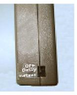
The LT-900 Long Range Transmitter has a switch to turn the transmitter on for instant or delayed operation or off to allow the caregiver to work with a patient and not have the alarm sound.
