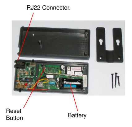
Remove the old battery from the battery holder and place the new battery with the positive end of the battery facing up towards the bottom of the unit towards the RJ22 connector. **BE SURE TO PRESS THE RESET BUTTON AFTER INSTALLING THE NEW BATTERY.**
