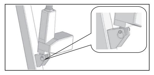
7. Attach the actuator bottom to the mast bracket and insert retainer pin, as shown above. Insert retaining ring through retainer pin hole to secure actuator base to mast bracket.
