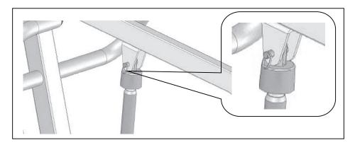
8. Attach the actuator top to the boom bracket and insert retainer pin, as shown above. Insert retaining ring through retainer pin hole to secure actuator top to boom bracket.
