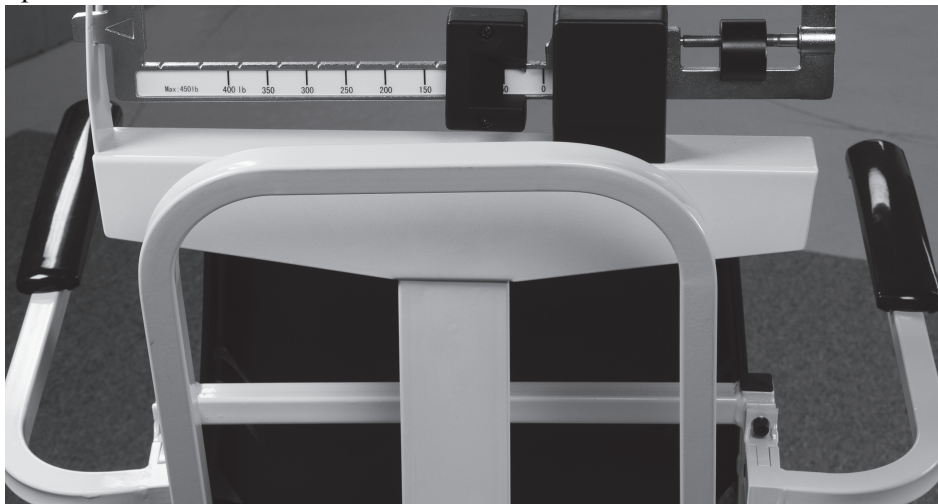
Figure 2-17. Secured Arm Rests
