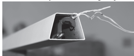
Figure 2-5. Remove Twist Tie from Steelyard Rod
