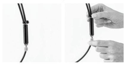
**15** Turn the thumbscrew counterclockwise to tighten the brake or clockwise to loosen the brake. When done, tighten the adjustment nut back to the brake adjuster housing without turning the thumbscrew.
