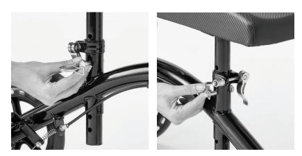
6 Insert the Seat Height Adjust Pin into the hole. Lock pin in place by sliding the loop over the protruding end of the pin.
