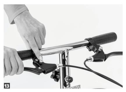
To lock the brake, squeeze and hold one of the hand brake levers to the Hand Grip and push and hold down the spring loaded push button (located on top of brake). Release the hand brake lever. When done correctly, push button with remain down and the hand brake lever will be locked in place. Rear wheels should not be able to rotate.
