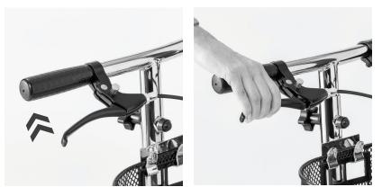
**12** To apply the brakes, simply pull one or both of the hand brake levers with your fingertips toward the hand grip. Either lever will operate the brake by itself.
