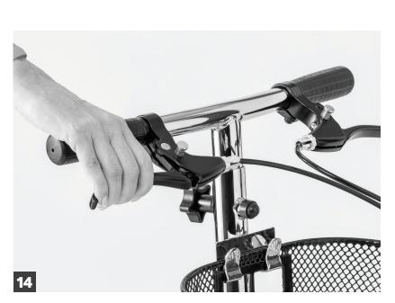
To release the brake, pull the lever towards the hand grip. Push pin will pop up automatically.
