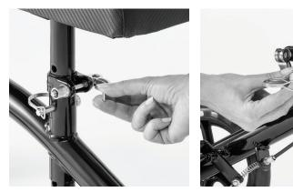
8 Loosen the Seat Cam Lock under the knee pad and remove locking pin.
