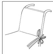
Tie the OneWaySlide to the rear frame tubing of the wheelchair.
