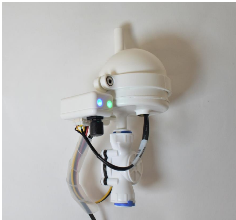
Figure 3-22: Flow Sensor Package with External Indicators
