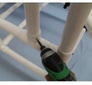
SECURE USING 1/2" RETAINING SCREWS. USING PILOT HOLES AS REFERENCE.
