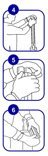
Don gloves. Place light where bulb is to be replace into an upright position that is comfortable to reach.
