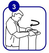
Gently turn the cone clockwise on the base. The cone should screw on smoothly, with little resistance. If you feel resistance, unscrew the cone, adjust its position slightly and try again until it screws on smoothly. Tighten until just snug. Don't overtighten. Unlock wheel caster to move unit.
