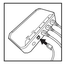
With both bases in FLAT position, connect each base to the other by inserting SYNC CABLE into each control box slot labeled sync.
