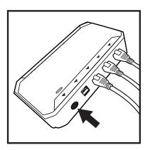
Double click the PAIR button on the control box (light will turn blue during the pairing process).
