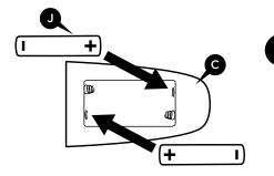
Lift the battery cover and insert the two AAA size batteries (included) into the remote as shown in the figure. Replace the battery cover. Remote is already linked with the base.
