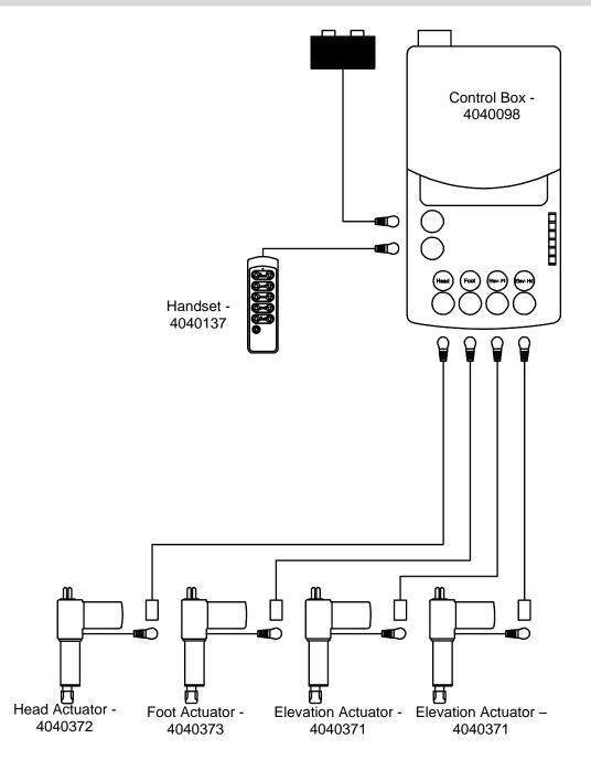
**NOTE:** To install Foot Board Control (4040148), a junction y cable is plugged into the control box instead of the handset, and the handset (4040137) and Foot Board Control cable (4040111) are plugged into the junction y cable. The Foot Board Control will get plugged into the Foot Board Control Cable.
