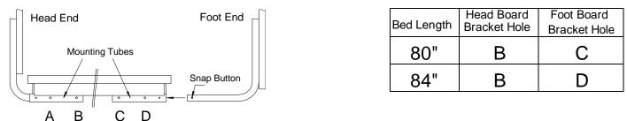
Normally the cap nuts are installed in the head and foot boards at the factory. If they are not installed at the factory insert the cap nuts provided in the hardware bag into the pre-drilled holes in the head and foot boards using a rubber mallet. If laminated on one side only, install the nuts on the laminated side of the board. Attach head and foot boards to the front face of the vertical bracket using the provided screws. Tighten all hardware.
