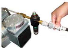
Quick-disconnect valve— "to compressor."
