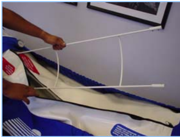
Side support being inserted into chamber opening
