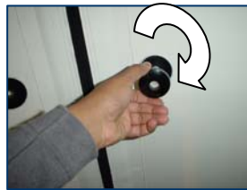
Fig. 16 Turn clockwise from inside to release pressure
