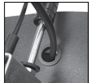
Insert Cable Connector Labeled SEAT Through Bushing
