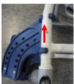
Step 3 Using an Allen wrench (A/F 5 mm), completely remove the screws (LH rotation) at the wheel units. When loosening the screws, press against the locking nut.
