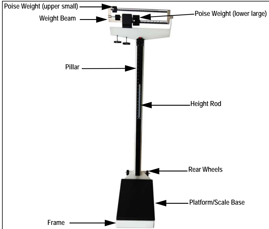
Figure 2-1. RL-MPS-40 Parts
