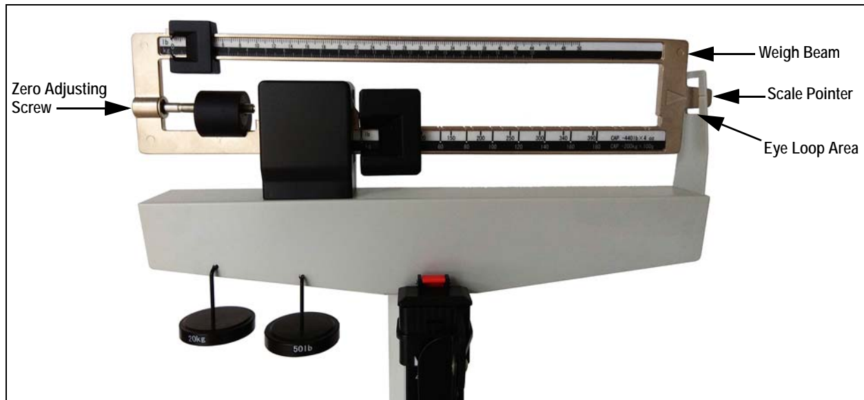
Figure 4-1. Eye Loop Area and Zero Adjusting Screw Location
