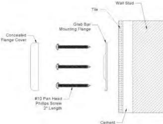
Apply a bead of silicone around the Grab Bar Mounting Flanges on the mounting surface to ensure a water-tight seal will be created at all mounting locations. Secure the grab bar to the wall using six (6) #10 Pan Head Phillips sheet metal screws (provided) and screw into the 1/8" holes created in the solid wood backing. Complete the grab bar installation by covering the mounting flanges with the Concealed Flange Covers, snapping them into place.
