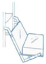
4. The Drop-Stop may be positioned to accommodate various degrees of ankle plantar flexion. This may be accomplished by securing the top straps to the upper section of the footrest support bars as shown in the illustration.
