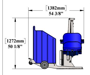
\*MEASUREMENT TAKEN WITH THE LIFT AT FULL LOAD\*
