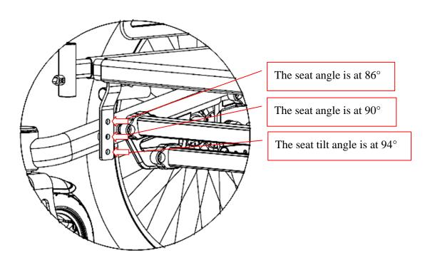
• The backrest angle can be adjusted according to the 3 adjustments below
