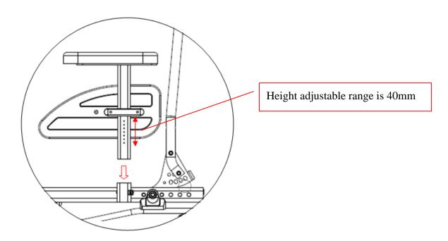
• The seat can be tilted and lowered according to the 3 adjustments below.
