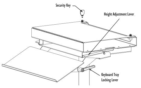
To open the cover and insert your computer, use the Security Key to turn the fasteners 1/4 turn counter-clockwise. The fastener should pop up to give a visible indication that it is unlocked. To refasten, use the key to push the fastener back into it's socket and turn clockwise until locked.
