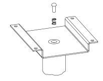
Place the Spring and Plunger into the recess in the top of the Upper Column Assembly
