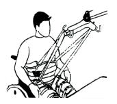
6a. Lower the carry bar of the ceiling lift to approximately the seated person's eye level height. Attach all four straps to the carry bar using loops of the same colour. Block the person's knees with a bed or frame. (Instructions also apply to fig. 6b). The sling is not suitable with all ceiling lifts. Please check with your supplier.
