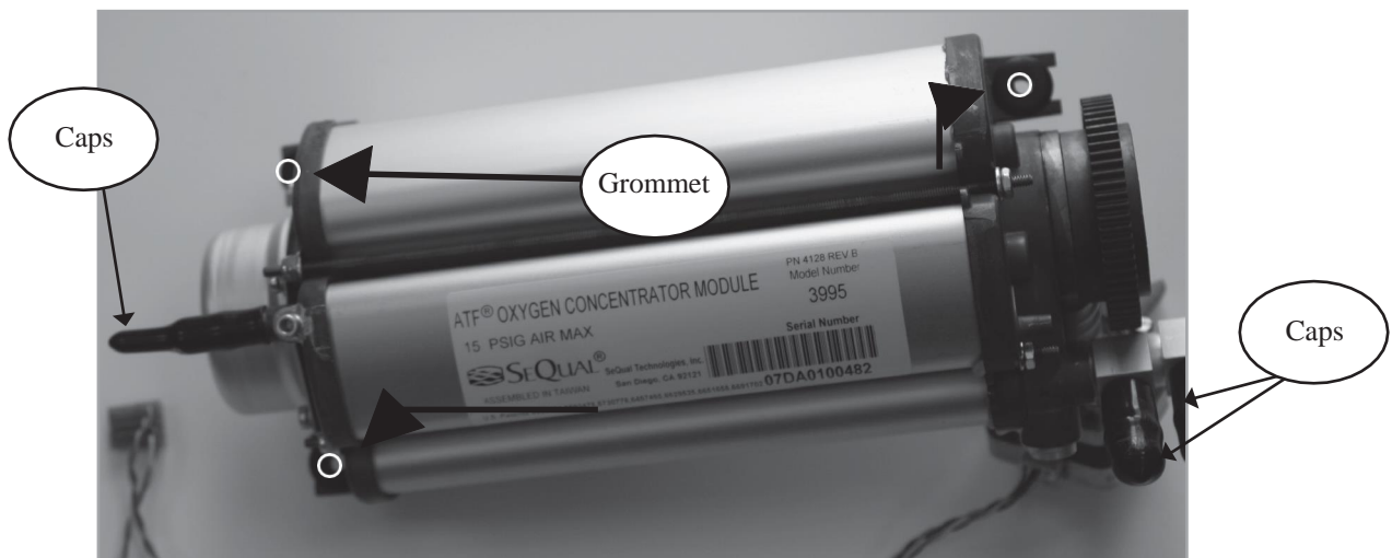
Figure 34: ATF Module Grommet Installation
