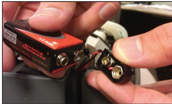
Figure 18: Disconnecting the 9-volt Battery.
