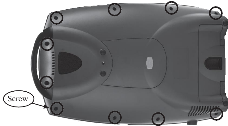
Figure 12: Removing screws to open the Front Cover
