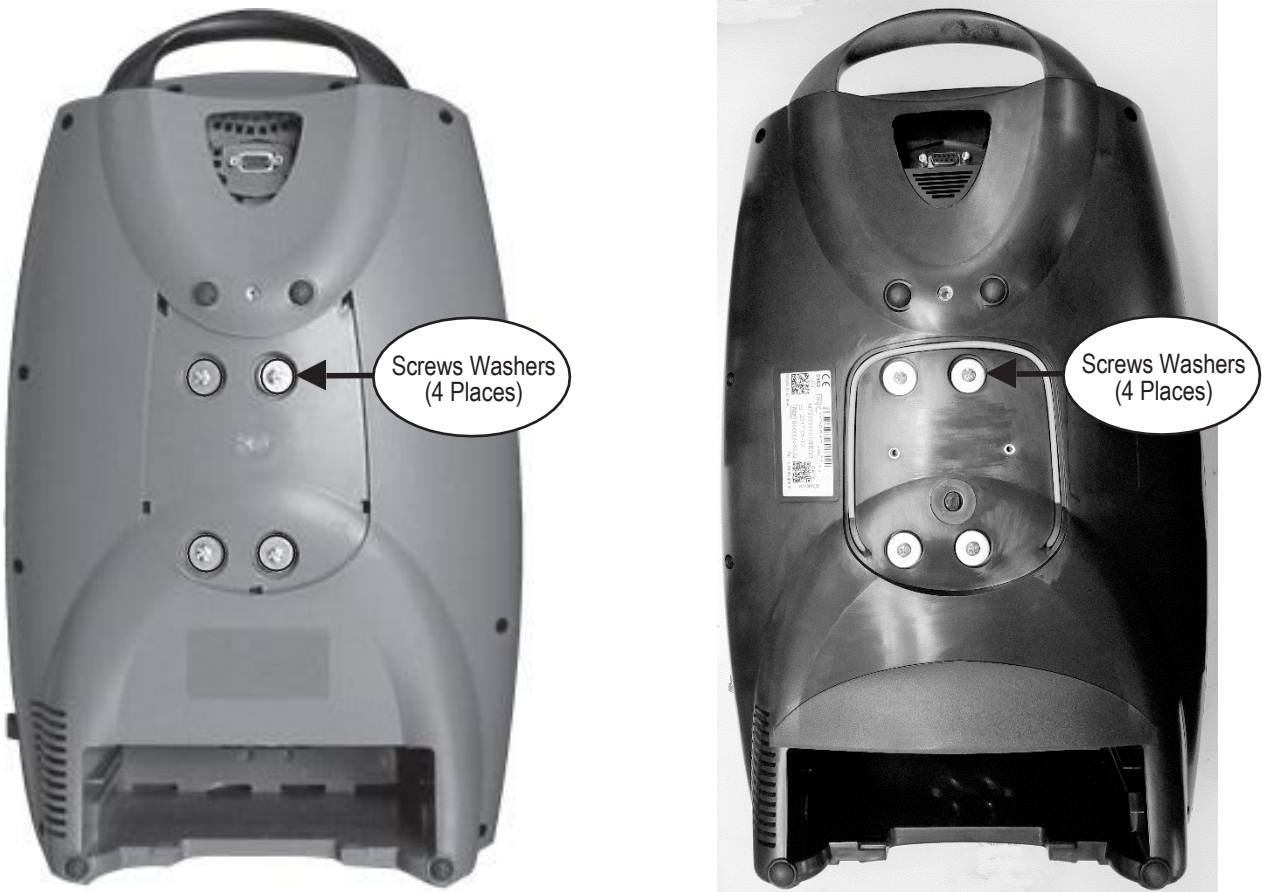
Figure 59: Remove Compressor Box screws.
