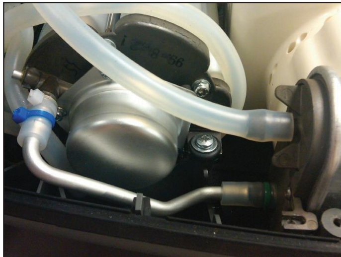
Figure 39: Product tank and hose barbs
