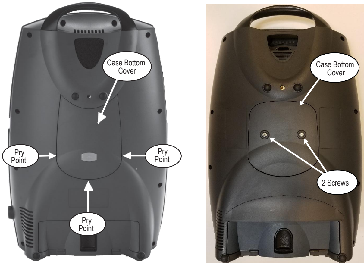
Figure 55: Case Bottom Cover Removal 3 LED model left photo, 2 LED model right photo
