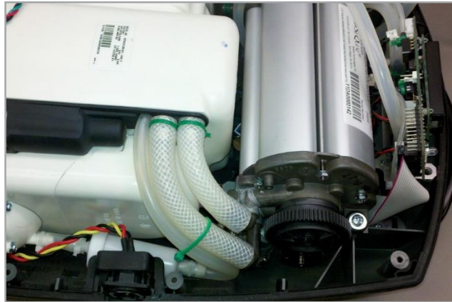
Figure 25: Installing the Compressor Intake Filter.
