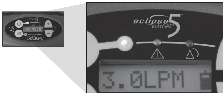
Figure 8: Power Cartridge Status Gauge (3 LED model pictured. 2 LED model does not have red LED.)
