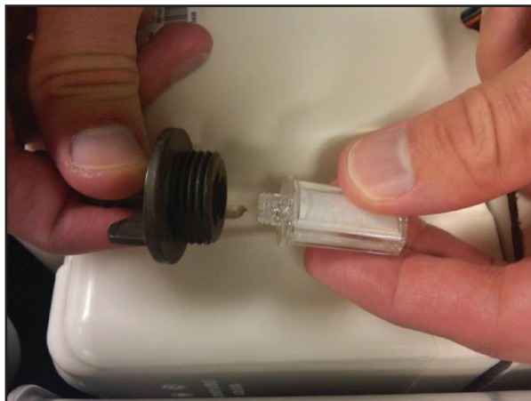
Figure 22: Installing the new HEPA Filter.
