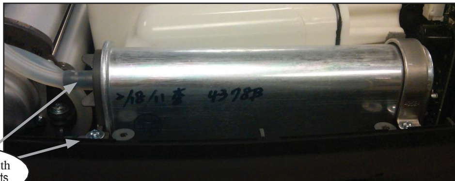
Figure 41: Connect output tubing
