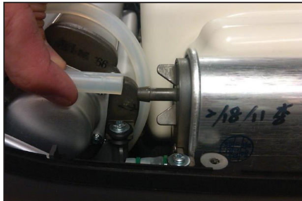
Figure 19: Tubing on Filter Carriage.
