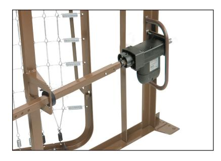
7. Hi/Low shaft connected to Hi/Low motor.
