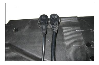
NOTE: Before installing motor, plug hand pendant and Hi/Low motor cable into motor as shown
