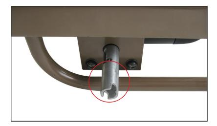
13. Release the spring loaded shaft on the hi/low motor and insert the shaft into the gear box on the footboard.
