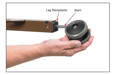
Install the casters by inserting the stem of the caster into the leg receptacle. It is recommended to install 1 locking caster and 1 nonlocking caster on each bed end. The locking casters should be installed diagonally from each other.
