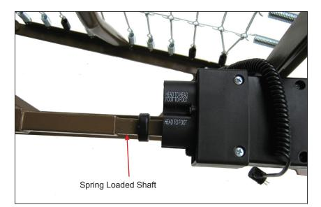
Install Hi/Low shaft to the Hi/Low motor at the foot section of the bed by inserting the spring loaded side of the shaft to the bottom receptacle as shown.
