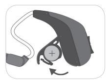
To power on, insert battery (+ side up) as shown and close the door. To power off, open the battery door.
