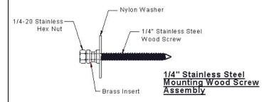
\*Above Items are Welded Together to Form Mounting Wood Screw Assembly.
