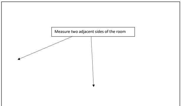
Based on these measurements, you will be able to select the best fitting rails for your room. Maximum coverage available is 23 ft by 23 ft and all setups must be rectangular/square. Minimum coverage is 14.1 ft by 9.02 ft.
