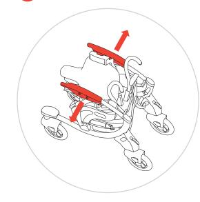
Unfold the Zeen by gripping and expanding the two side frame tubes near arm-rests. When mid-way expanded, pivot handlebars forward.
