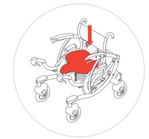
Next push down on seat until audible click confirms the seat is fully locked.
