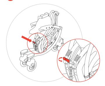
With the Zeen upright and wheels on the ground, remove protective plastic wrap. Then pull open the front Velcro folding strap. Rotate the straps vertical for easy use of the handlebars.
