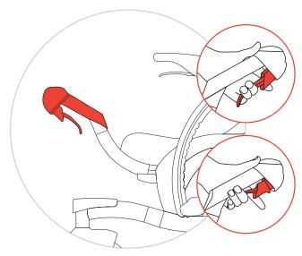
On the handlebars, fully squeeze the long coasting brake levers with middle, ring and little fingers, and add index finger (or your other hand) to pull up the short parking latches until they 'park' the brakes. Sit down on the Zeen seat.
