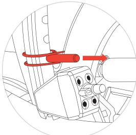
Remove the shipping pins from the frame tubing on both sides by freeing the elastic cord and then pulling the pin from the hole in the strut. Please retain these shipping pins for future use when transporting the Zeen.
