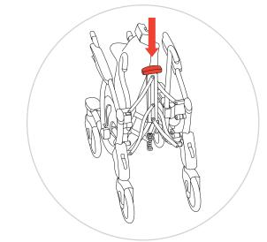
Push down on the red rear folding handle and lock into expanded position.
