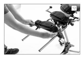
13. If the independent adjustable calf pads were ordered, loosen the ratchet handles on the clamps and position as shown. Insert the calf pads into the inside of the clamp. Tighten securely.
