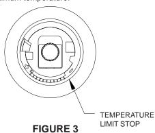
The main handle of the Temp-Gard III valve is for temperature control only. To turn valve on, the handle is turned counterclockwise through the cold position, to the warm and then to the hot position. The range of motion on the
